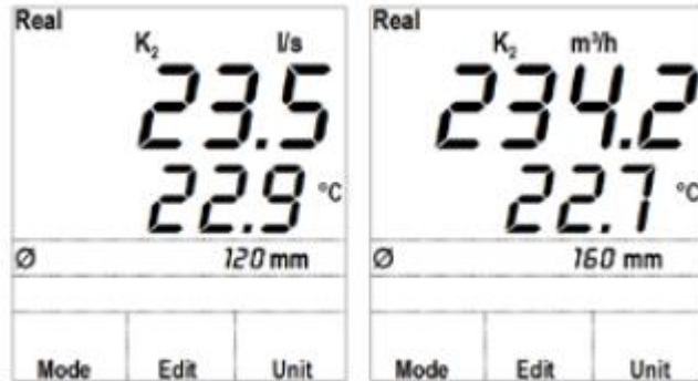
Air flow measurements in l/s and m 3 /h and given diameters
