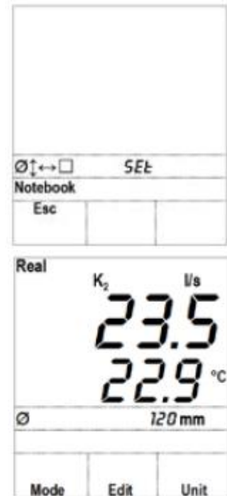
Air flow measuring with given diameter
