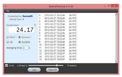
With SwemaTerminal 3 it's possible to measure with a single probe. You can also do online logging and store the logged data on your PC, update firmware, print calibration protocol and change settings. Information of what kind of probe and at which COM-port it's connected can be found on the top left side.
