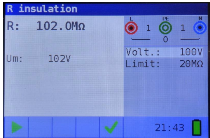
Figure 5-3 Example of insulation resistance measurement results
