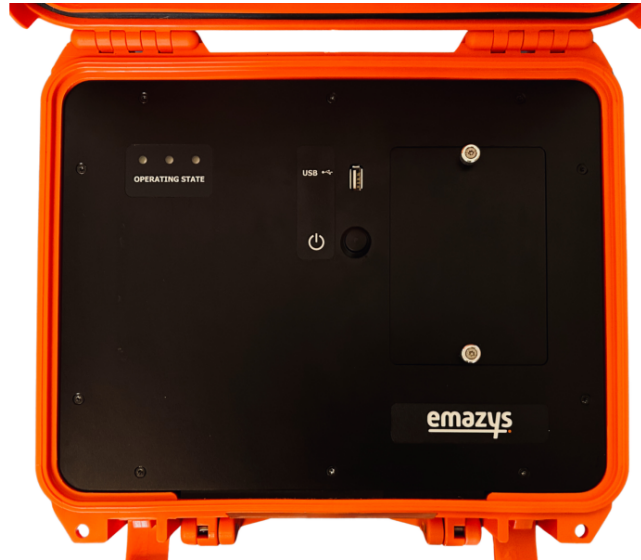
Figure 1: Z300 PVT front panel. Placed on the middle of the front panel we find the ON/OFF switch. When the instrument is turned on a small LED in the button will emit green light. The instrument USB connector is found above the ON/OFF button. This connector can be used for various purposes such as software updates etc.
