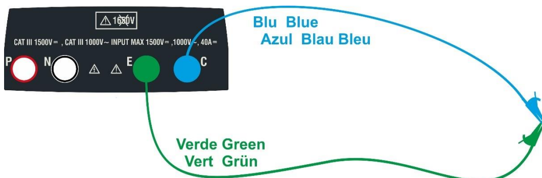
Fig. 5: Compensation of the measuring cables resistance
