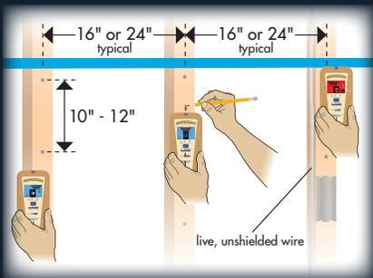
While still holding the Power Button, from the stud center indication, slide unit VERTICALLY. TC™ will identify the screws and plates on top of the stud and the clean, ‘safe-to-drill’ zones in between.
