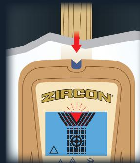
Continue sliding. When target center is detected, target icon displays and SpotLite® Pointer illuminates. Mark this location.
