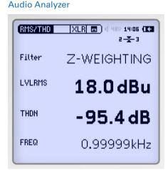
The XL2 with balanced XLR and unbalanced RCA inputs offers a comprehensive, high performance audio analyzer. It simultaneously measures balance, level, distortion (THD+N) and frequency.
