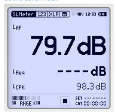
The XL2 provides a precise sound level meter for events and environmental noise monitoring. Numerous measurement variations are simultaneously available. Actual level, Lmin, Lmax, Leg may be measured in combination with frequency weighting A, C or Z and time weightings fast, slow and optional impulse. All results are simultaneously available.
