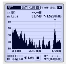
The real-time FFT is the ideal tool for visualization of comb filters and narrow band effects. It measures the actual level and the averaged level Leg in three ranges over the entire audio band.
