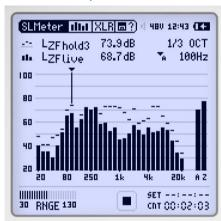
The RTA perfectly suits tasks such as optimization of sound systems and rooms. The XL2 measures and logs wideband values and the real time spectrum in 1/1 or 1/3 octave-band resolution.
