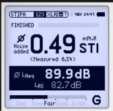
The XL2 Analyzer measures the speech intelligibility according to the latest revision of standard IEC 60268-16. It offers ambient noise correction and automated averaging for repeated measurements. The XL2 displays the speech transmission index (STI) and the common intelligibility scale (CIS), accompanied by the individual levels and modulation indices of the seven octave bands.
