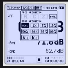
The Extended Acoustic Pack supports the daily tasks of acoustic consultants. It offers additional features for sound level logging and acoustic measurements, such as recording linear wav-files, percentile statistics, sound exposure level, 100 ms logging, event monitoring, RT60 in 1/3 octave resolution, Zoom-FFT with 0.4 Hz resolution and many more.
