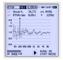
Measure the energy decay with automated triggering using an impulse signal or gated pink noise as signal source, and determine if the room fulfills the RT60 requirements.
