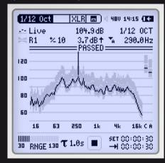
The Spectral Limits Option adds an RTA Analyzer with 1/6 and 1/12 octave spectral resolution and the Zoom-FFT. It extends the XL2 function range with trace capturing, relative curve display and comprehensive tolerance handling. The XL2 Analyzer compares spectral measurements against reference curves or a tolerance band including PASS/FAIL results.
