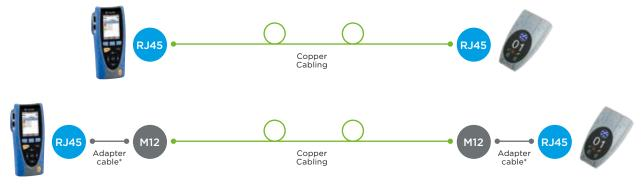
2 x M12 D connector cables supplied as standard. M12 X connectors available as accessories.
