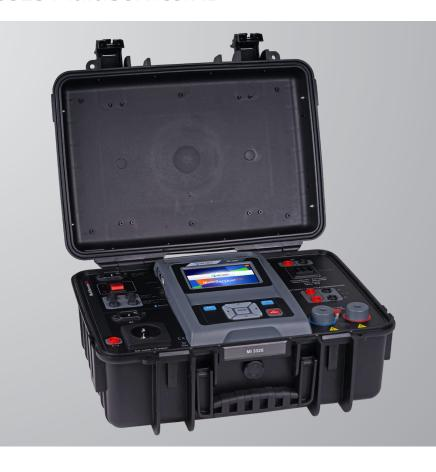
is a top-of-the-line multifunctional instrument covering diverse industrial applications, where ruggedness and reliability are a must. In Metrel range of the instruments it is introduced as a successor of MI 3321 MultiServicerXA. The new platform integrated in the MI 3325 MultiServicerXD features support for colour touch screen technology, advanced memory organizer including large SD card storage media and state of the art AUTOSEQUENCE®s.
