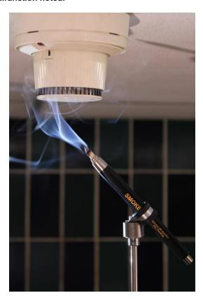
We do now provide two adapters that fit our telescopic tool, these adaptors is manly developed for our products SMOKE-PEN and smaller smoke emitters such as AX-5 &13 and our 1-9 gram encapsulated products.
