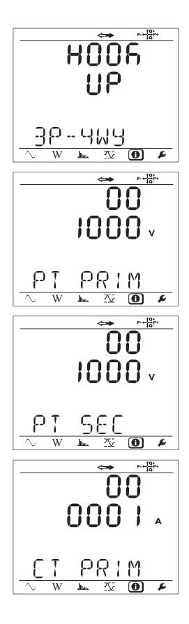
Nominal primary current of the neutral (if a sensor is connected to the I<sub>N</sub> terminal)
