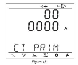
Depending on the type of current sensor, MiniFlex®/AmpFlex®, MN clamp, or adapter unit, enter the nominal primary current. To
