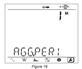
To change the aggregation period, press the **Enter**  $(\frown)$  key, then use the  $\blacktriangle$  and  $\triangledown$  keys to choose the value (1 to 6, 10, 12, 15, 20, 30, or 60 minutes).
