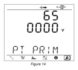
To change the nominal primary voltage, press the **Enter**  $(\bullet)$  key. Use the  $\blacktriangle$ ,  $\blacktriangledown$ ,  $\blacktriangle$  and  $\triangleright$  keys to choose the voltage, between 50 and 650,000 V. Then validate by pressing the **Enter**  $(\bullet)$  key.
