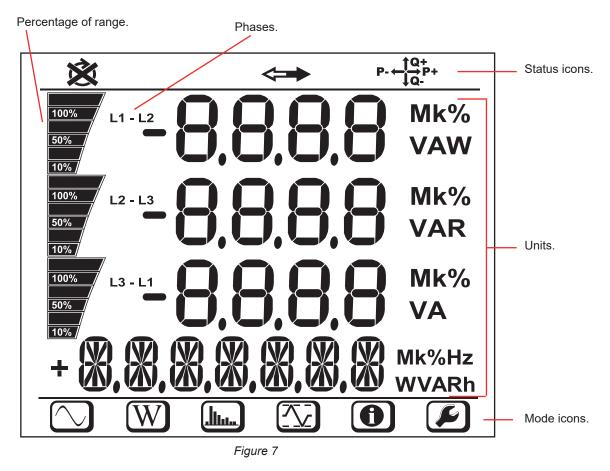
When there is no user activity for 3 minutes, the backlighting is switched off. To switch it back on, press one of the navigation keys  $(\blacktriangle \lor \blacklozenge \triangleright)$ .
