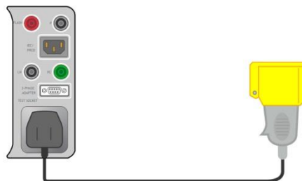
Figure 9.2: Connecting 110 V Test Adapter (A 1474)
