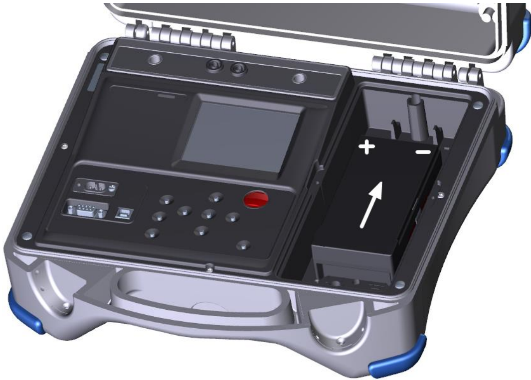
Figure 7.2: Correctly inserted battery
