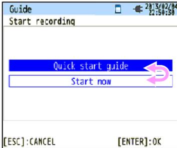
Press the **Cursor** Key to move the **blue highlight**, showing the item is being selected, over the items in blue letters. In the screen at the left is the Recording start screen. Press the **Cursor** Key and move the blue highlight on the desirable recording method, and press the **ENTER** Key to confirm the selection. To quit the start guide, press the **ESC** Key.
