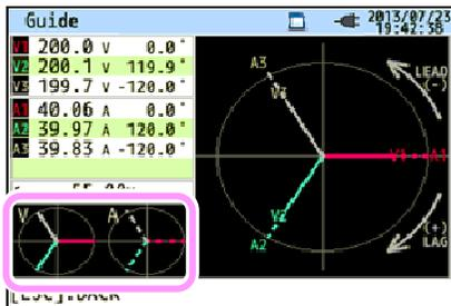
Close the result display. Then, the blinking vectors and the values of NG items will be displayed. If all the results are OK, the ideal vector diagram will be displayed at the lower left corner.
