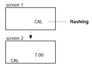
4) Place the electrode into pH 7.00 buffer solution (PH-07A) Press the "Hold button" (3-3, Fig. 1) once. The "7.00" will flashing, following show "End". then return the normal measurement screen and finish the pH 7.00 calibration procedures.
