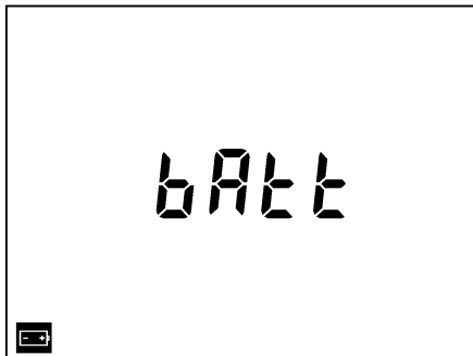
Figure 5: The low battery indicator signals the need for a replacement.
