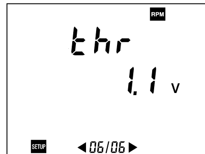
Figure 54: Display of parameter relating to the threshold voltage of the tachometer sensor.
