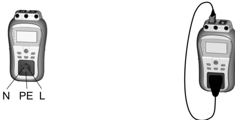
**Figure 5.25:** Polarity test of IEC cord
