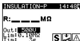
**Figure 5.12:** Insulation resistance - P menu
