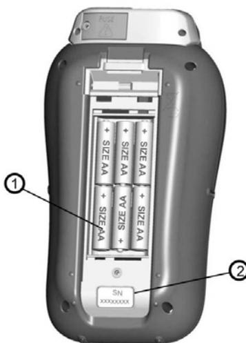
Figure 2.4: Battery compartment
