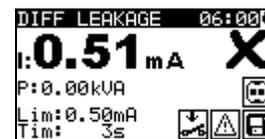
**Figure 5.29:** Examples of differential current measurement result
