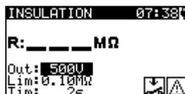
**Figure 6.29:** Insulation resistance starting screen
