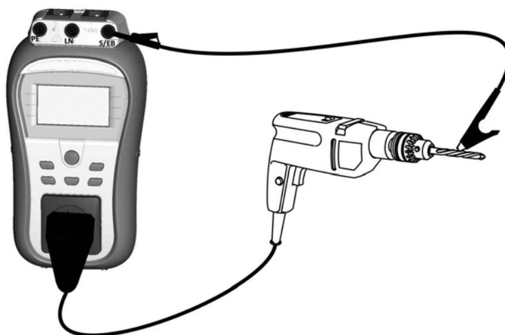
**Figure 5.13:** Measurement of Insulation resistance - P
