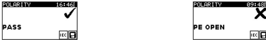
Figure 5.26: Examples of polarity test result
