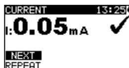
**Figure 6.48:** Clamp current result screen
