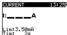
**Figure 6.47:** Clamp current starting screen
