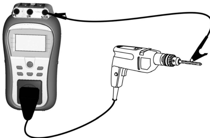
**Figure 5.21:** Measurement of Substitute leakage - P current
