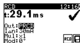
**Figure 5.37:** Examples of (P)RCD single test results
