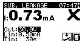
**Figure 5.19:** Example of substitute leakage current measurement results
