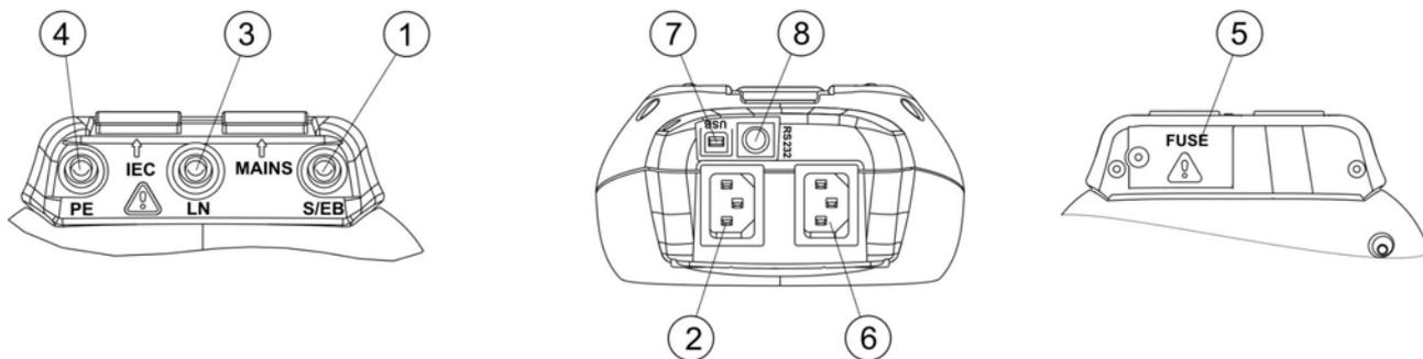
**Figure 2.2:** Connector panel
