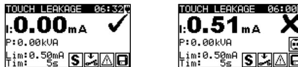
Figure 5.33: Examples of touch leakage current measurement results
