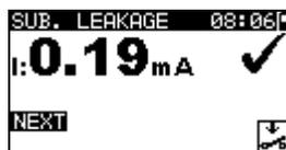
**Figure 6.32:** Substitute leakage result screen
