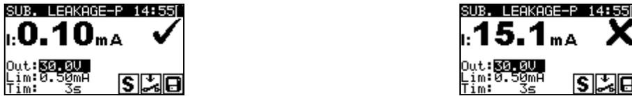
**Figure 5.23:** Example of substitute leakage - P current measurement results
