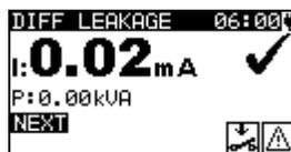
**Figure 6.34:** Differential leakage result screen
