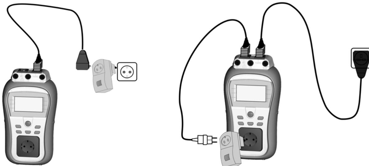
b) Testing of PRCD via mains socket
