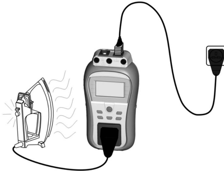
**Figure 5.39:** Power test
