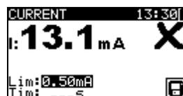
**Figure 5.45:** Examples of clamp current measurement result
