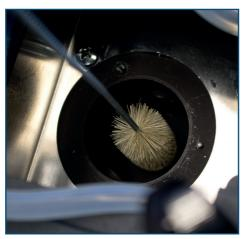
12. Clean with a pipe cleaner the connector of the heated line to the measuring chamber. (For technical reasons, it may be for some devices, this is not possible.)
