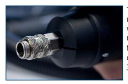
15. Clean sealing coupling regularly with a cloth and grease it with resin-free oil.Clean the dust duct from time to time with water, after that dry the dust duct with compressed air (max. 3 bar).
