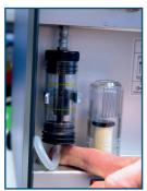
1. Loosen the water trap out of the holder
