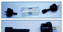
3. The cylinder from the upper part unscrewing and check the holes and the input and output, and if necessary, clean with compressed air.
