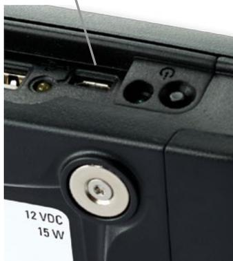
The micro USB port on the DG-1000 can be used to create a wired two-way communication link between the gauge and a Windows computer. Use of the micro USB port requires you to first download and install the appropriate USB Device Driver to the computer using the Windows Update service.
