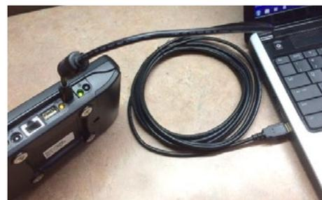
TEC software installed on the PC will now be able to detect the gauge and create a communication link. The gauge and computer can be located up to 16 feet from each other when using a USB cable.
