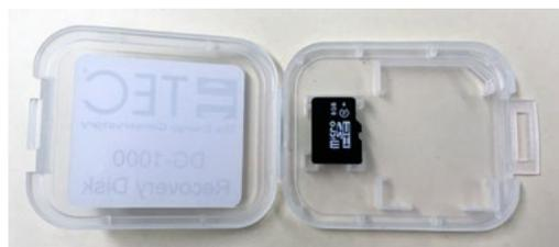
The recovery disk is a micro-SD card that should be used only if you need to reset the DG-1000 to the factory settings. If a situation arises where the recovery disk may need to be used, consult with TEC technical support first by calling 612-827-1117.
