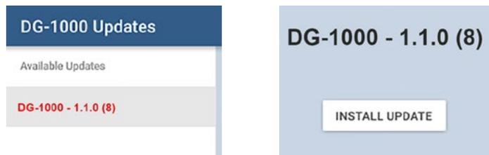
9. After touching Install, the following message will appear: *"Install package? The current package will be removed and replaced with 'package name.' A device reboot will be required. Please ensure the gauge is plugged into its charger before continuing."* Touch OK to proceed. When the update is complete a message will appear that says *"Power off. The device will power off to complete the update."* Touch Power Off to complete the update process.
