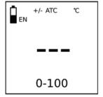
If the display appears as below, it means the instrument is in external measurement mode. To revert back to the internal measurement mode, switch the unit off, and then remove the attached external probe.
