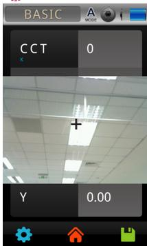
3 A viewport will display on the screen with a "cross hair" mark in the middle. Press the "Measure" button on the left side at appropriate distance.
