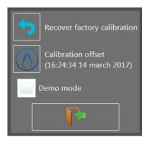
You can easily calibrate the recorder inputs for the voltage and thermocouple offsets. This will remove any offset present on different channels.
