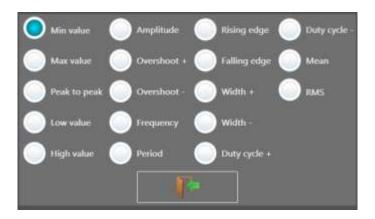
18 various mathematical formulas are available. You can display up to **5 simultaneous calculations** on screen The display is made in windows above the diagrams, where are specified:
