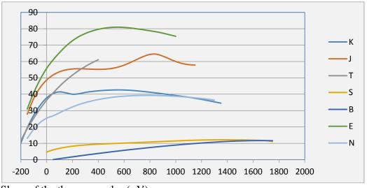
Slope of the thermocouples  $(\mu V)$
