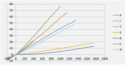
Tension of thermocouple (mV)
