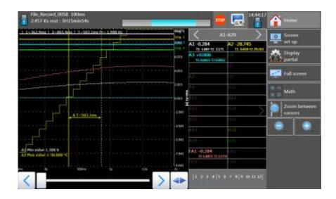
When waiting for the trigger, the screen makes it possible to display the channels in real time (scrolling mode); you can select the scrolling rate.
