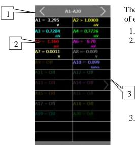
The numerical window allows to visualize in real time the values of each channel.
