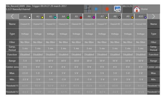
This table gives you a quick insight of the various adjustments of the channels. You can change these adjustments directly in this table by pressing the parameter you want to update. You can display 10 channels maximum.
