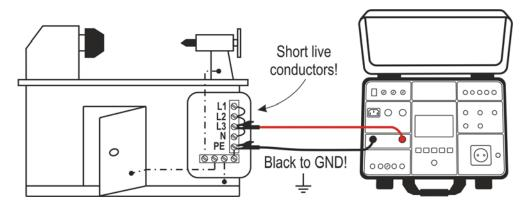
Figure 12: Connection of test leads
