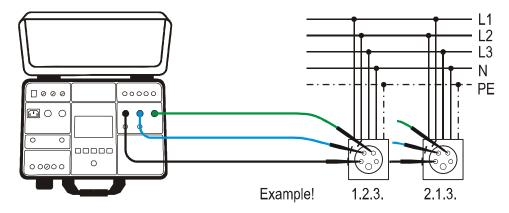
Figure 40: Connection of test leads in PHASE SEQUENCE measurement
