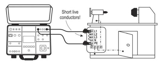
Figure 17: Connection of test leads
