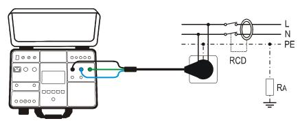
Figure 24: Connection of test cable to schuko socket for LOOPL/N or LOOPL/PE measurement
