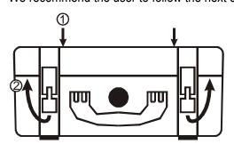
Figure 1: Opening the instrument's cover
