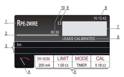
Figure 4: Basic measurement screen in RPE-2WIRE function
