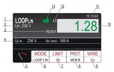
Figure 23: Display with LOOPL/N test result
