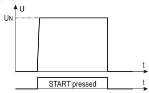
Figure 14: Presence of test voltage with regard to pressed START button in MANUAL or BURN mode
