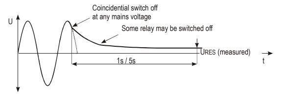
Figure 32: Discharge diagram in non-linear circumstances
