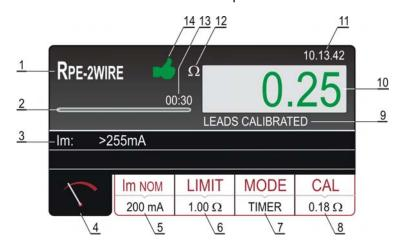
Figure 5: Display with RPE-2WIRE test result
