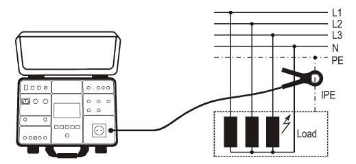
Figure 45: Connection of current clamp in ILEAK measurement, CLAMP mode
