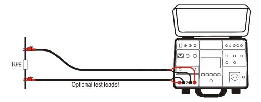
Figure 10: Connection of optional Kelvin test leads
