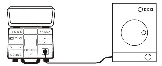
Figure 38: Connection of UUT to schuko test socket
