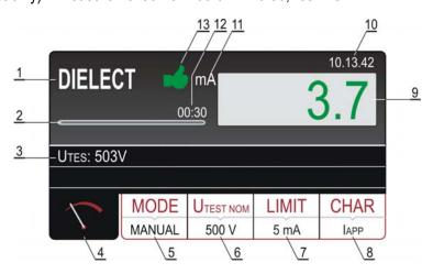
Figure 13: Display with DIELECTRIC test result
