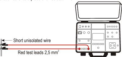
Figure 6: Connection of test leads for calibration purpose
