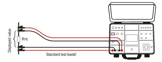
Figure 9: Connection of standard test leads
