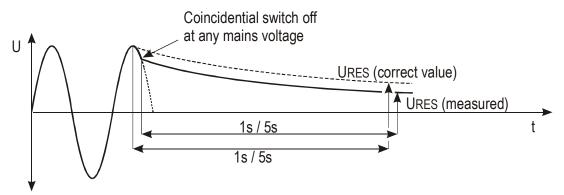
Figure 31: Discharge diagram in linear circumstances
