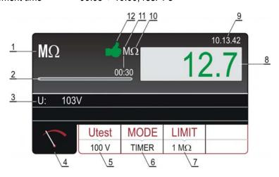
Figure 11: Display with RISO test result
