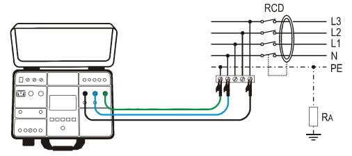
Figure 22: Connection of test leads
