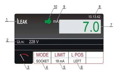
Figure 44: Display with ILEAK test result in SOCKET mode
