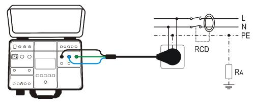
Figure 21: Connection of schuko test cable
