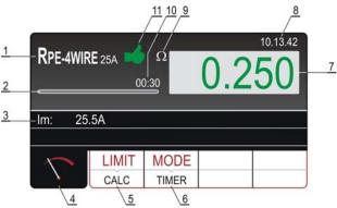
Figure 8: Display with RPE-4WIRE test result
