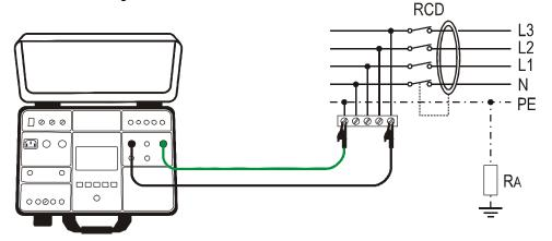
Figure 30: Connection of test leads to tested wiring
