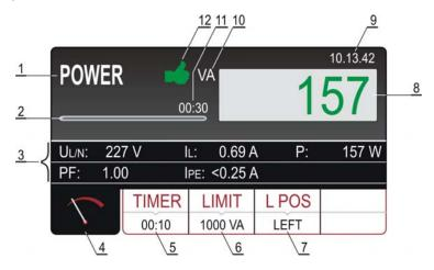
Figure 37: Display with POWER test result
