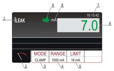
Figure 43: Display with ILEAK test result in CLAMP mode
