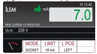
Figure 69: ILEAK function RECALL screen
