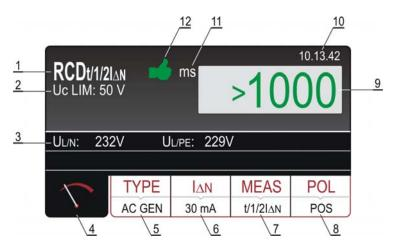
Figure 18: Display with RCD test result
