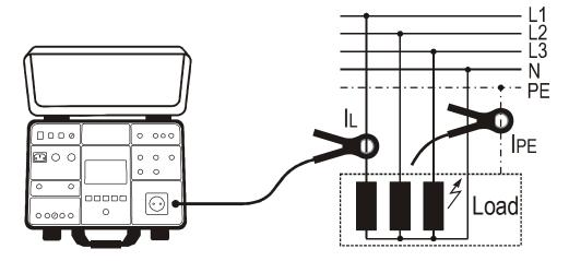
Figure 42: Connection of current clamp in ICLAMP measurement
