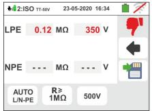
Press the **SAVE** key or touch the icon is for the partial saving of the test and to <u>end the test sequence</u>. The instrument shows the message shown in the followed screen for a few seconds
