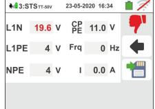
44 If the test fails, the screen like the one on the side is shown on the display. The incorrect value of the parameter is shown in red and the symbol **r** indicates
