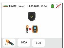
2. Connect the clamp T2100 by inserting the connector into input **In1** of the instrument. Turn the clamp on and put it in "RS232" mode (see the user manual of the clamp). The
