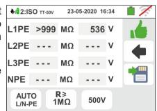
14 Connect the input **B1** on the input **L2** of adapter as shown in the screen to the side
