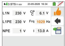
32 If the test fails, the screen like the one on the side is shown on the display. The incorrect value of the parameter is shown in red and the symbol **r** indicates
