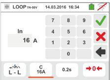
Move the slide bar reference by selecting the protection tripping time between the options: 0.1s, 0.2s, 0.4s, 1s, 5s (all countries except AUS/NZ and UK), 0.4s, 5s (option L-PE, Fuse protection for AUS/NZ and UK) and 0.4s (option L-PE, MCB protection for AUS/NZ).
