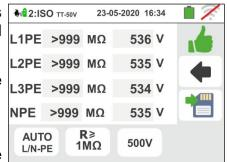
17 The measurement result of the L3PE and NPE test is shown in the screen to the side. The values of the real test voltages are shown on the display
