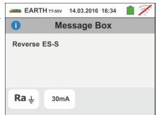
2. When starting a measurement, the instrument checks the continuity of measuring cables. If the <u>voltmetric</u> circuit (red cable S and green cable ES) is interrupted or its resistance value is too high, the instrument displays a screen similar to the one on the side.
