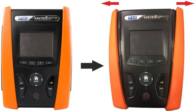
Fig. 40: Remove lateral half-shells
