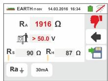
9. For <u>earth resistance measurement in TN systems</u>, in case of **positive** result (measured value LOWER than set limit value), the screen to the side is displayed by the instrument. It contains also the value of contact resistance of the voltage probe (Rs) and the value of contact resistance of the current probe (Rh).
