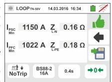
Press the GO/STOP key <u>for few seconds</u> or the START key on the remote lead. During this whole stage, do not disconnect the measuring leads of the instrument from the system under test.
