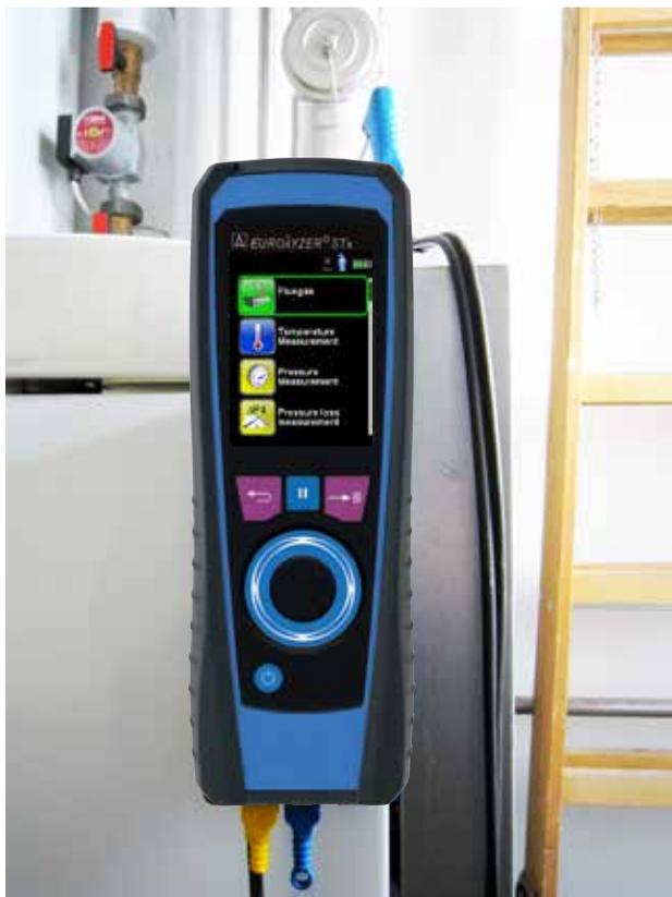
There are a variety of data interfaces, such as USB, Bluetooth Smart (BLE), infrared and MicroSDHC card for communication with other devices, PC or the EUROprinter available.
