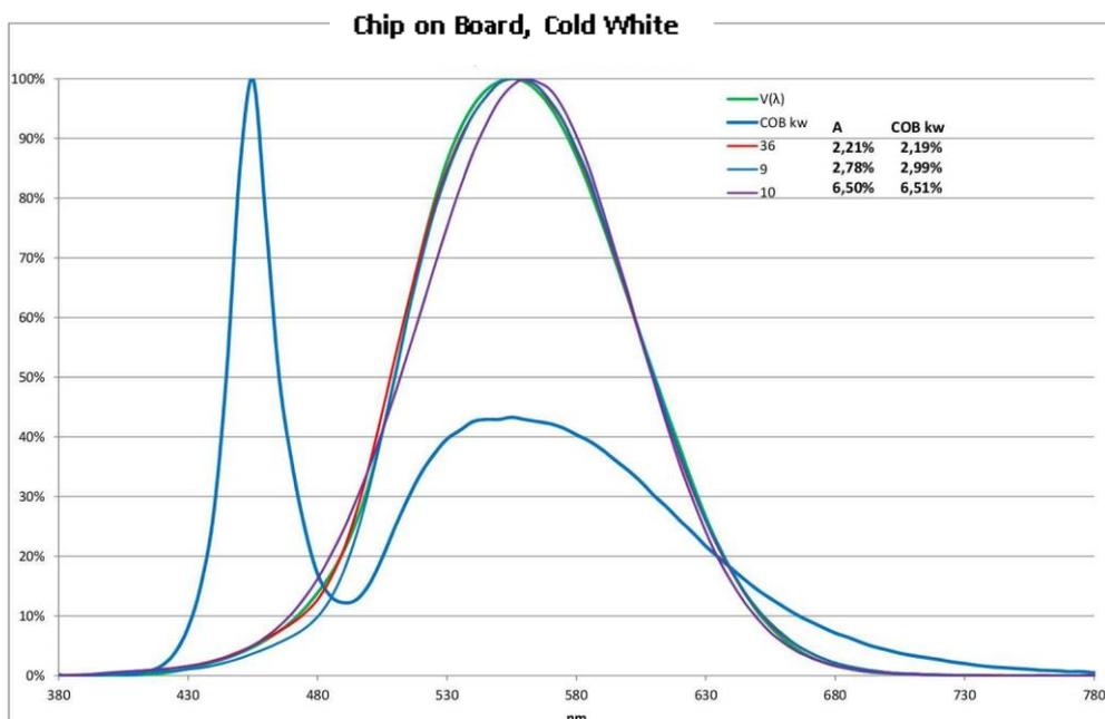
With this LED as well, f1 error remains unchanged. It's practically identical to error for light type A with all three filterings.
