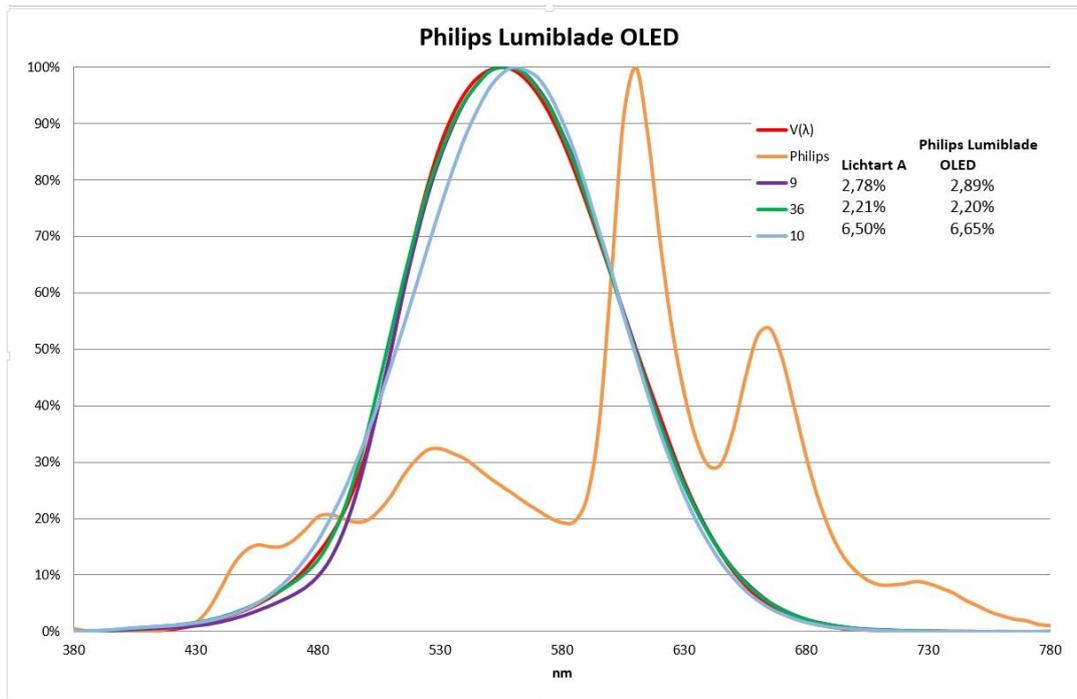
As with all LEDs that are used for lighting purposes the error relative to light type A is not yet significant.
