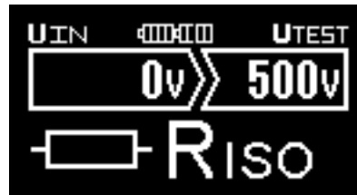
Fig. 3.5 Example of setting for insulation resistance measurement
