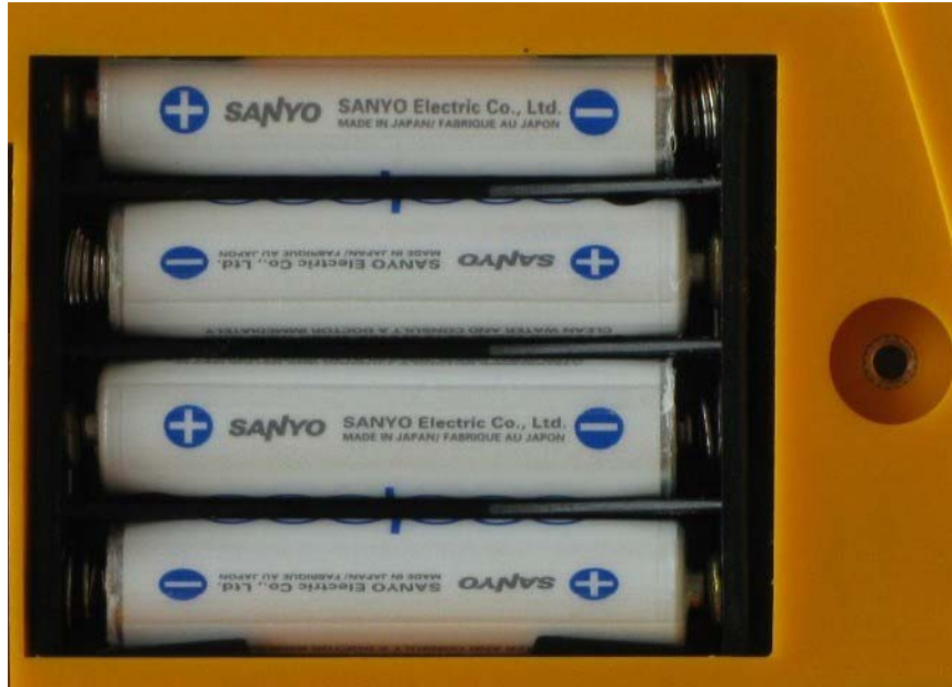
Fig. 4.1 Correct batteries/accumulators polarity
